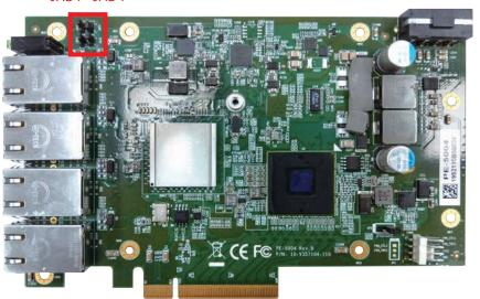
PE-5004 controls PD69104B PoE Power ON/OFF via SMBUS. Jumper JAD1~ JAD14 address setting as below (1-2=H, 2-3=L):
