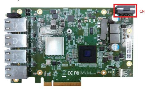
The PE-5004 is also equipped with one 4-pin power plug (12V, 6A max) for additional power supply. For most cases, the power obtained from PCIe bus is sufficient for the PoE devices, and you do not need to supply extra power to the card.In case the external power is needed, you can use 4-pin ATX power connector (+5V/Red, GND/Black, GND/Black, +12V/Yellow) inside the host computer. Please always confirm the polarity before you plug into the onboard 4-pin power plug.
