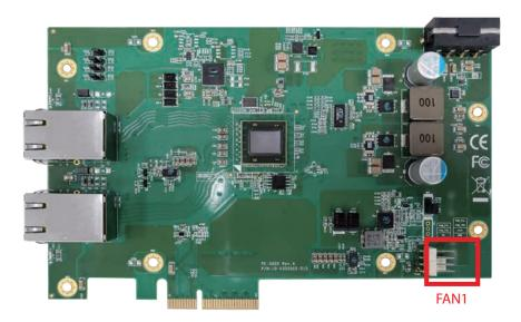
Fan power connector supports for additional thermal requirements. The pin assignments of FAN1 is listed in the following diagram :
